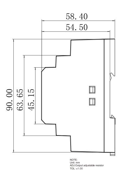
ADMISSIBLE DIN-RAIL:TS35/7.5 OR TS35/15 Terminal Pin No. Assignment
